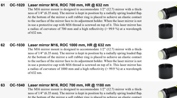
At the bottom of the mirror a soft rubber ring is placed to achieve an elastic contact to the surface of the mirror face to its adjustment holder. When the laser mirror is not in use a protective cap with M16 thread is screwed on top of it. This laser mirror has a radius of curvature of 700 mm and a high reflectivity (> 99.9 %) at a wavelength of 1180 nm.
